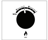
4. To increase the Water Temperature, turn the GAS Control to WINTER MAX and allow the temperature to stabilise. Note: Winter Max is shown on the dial and is different to summer Max.
