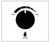
Adjusting the Water Flow will also help to achieve the desired Water Temperature (i.e. The higher the flow rate - the cooler the water will be. The lower the flow rate the hotter the water will be). NOTE: The unit will switch off automatically if the water temperature exceeds 50°C.
