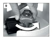
Connect the hose adaptor to the outlet on the gas cylinder. Turn the cylinder on in an anti-clockwise direction one (1) full turn. Check all LPG connections for leaks with a solution of soapy water (do not use a flame).
