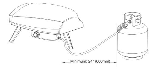
Only use the appliance with gas cylinder that does not exceed 600mm in height and 300mm in diameter.
