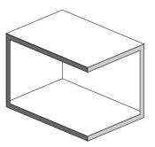
Within a partial enclosure that includes an overhead cove and no more than two walls. A common example is an outdoor gazebo.
