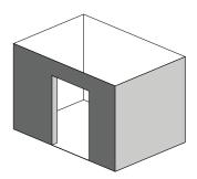
An enclosure with walls on all sides but at least one permanent opening at ground level.
